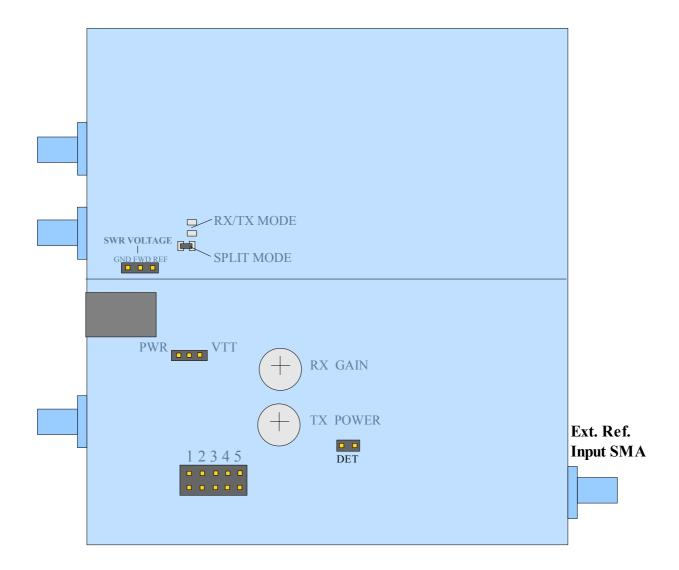
Ext. Ref. Input SMA - Input for optional external high stability reference oscillator, switchable by Jumper 5
